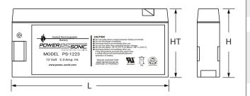
**L:** 7.17 (182) **W:** 0.94 (24) **H:** 2.40 (61) **HT**: 2.40 (61) Tolerances are +/- 0.04 in. (+/- 1mm) and +/- 0.08 in. (+/- 2mm) for height dimensions. All data subject to change without notice.
