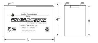
Tolerances are +/- 0.04 in. (+/- 1mm) and +/- 0.08 in. (+/- 2mm) for height dimensions. All data subject to change without notice.
